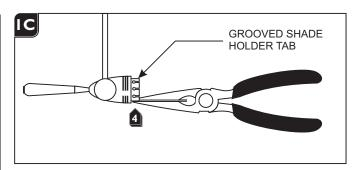
If the Prism glass shield fits tight onto the fixture, then carefully bend the grooved shade holder tabs in slightly with the needlenose pliers. If it fits loose, then carefully bend the grooved shade holder tabs out slightly with the needlenose pliers.
