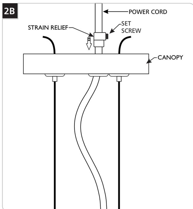
NOTE: The power cord does not support the fixture. For a casual "lazy cord" look, cut the power cord several inches longer than the drop height of the fixture.
