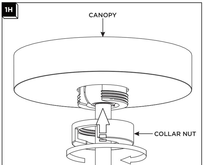
**10** Raise the canopy up until it touches the ceiling, and then tighten it down with the collar nut. For the slotted nut, turn until the slot aligns with the slot in the screw collar's cradle.
