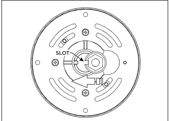
**9** Lift the fixture straight up, so that the ball rests in the cradle. Note: orientation needs to be aligned with the slot on the ball. Ensure any wire slack is kept above the screw collar, so that wires do not pinch.
