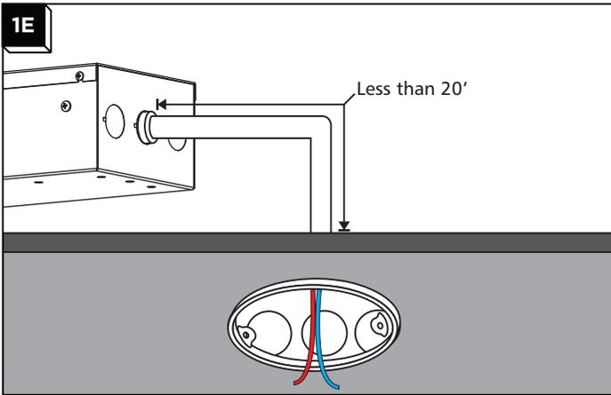
**6** Feed wires through conduit to remote driver location. Ideally, no farther than 20' from the fixture.
