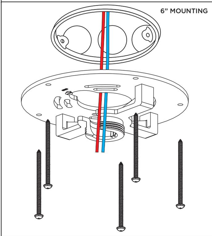
**7** For the 5": Screw the mounting plate to a standard j-box with the supplied screws.
