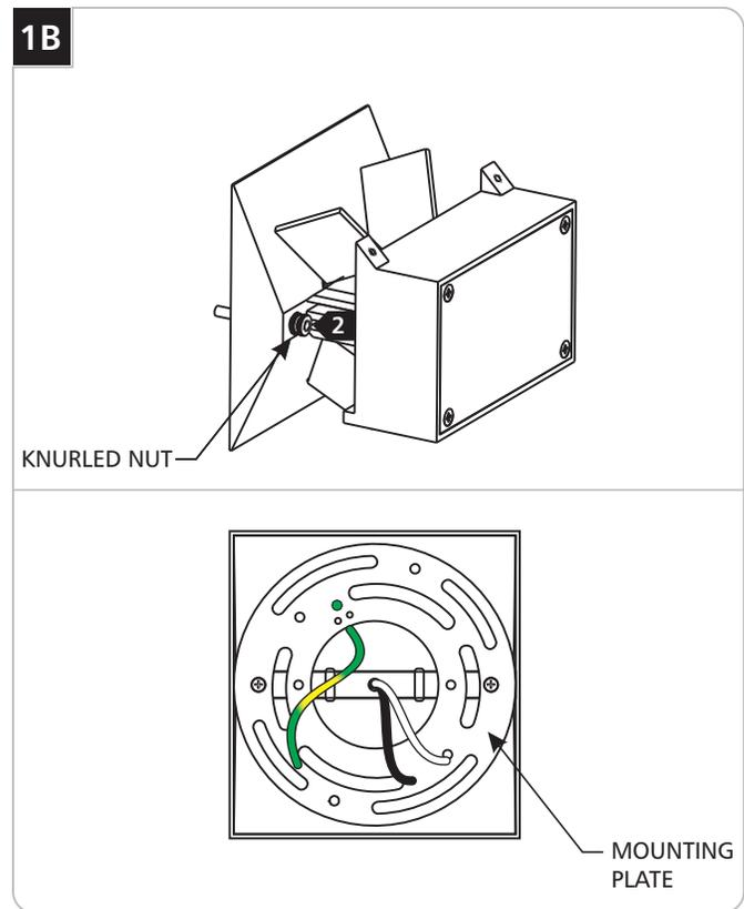
**2** Unscrew and remove the knurled nuts.
