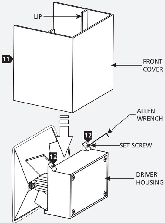
**NOTE:** Make sure the sealant is dry before reinstalling the cover.
