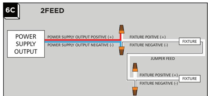
**NOTE: 2FEED fixtures are supplied with a jumper that can be used to power fixtures further down the run, that are separate from the initial run.**
