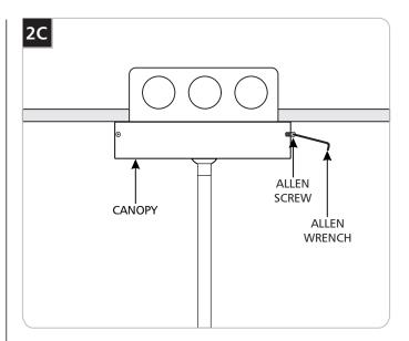
Place the drivers, all wires, and wire nut connections properly inside the canopy, place the canopy flush onto the ceiling, and secure it by reinstalling the three Allen screws with the provided Allen wrench.
