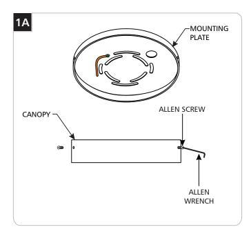
1 Separate the mounting plate from the canopy by unscrewing the three Allen screws using the provided Allen wrench.
