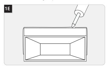
**10** For wet location installation, caulk around the mounting base with waterproof construction sealant.
